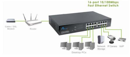
Your network device (i.e. computer, switch, IP Camera, VoIP) can be connected to any port of the Switch via a two-pair Category 5 Cable or above. If the LED indicators do not light up after making a proper connection, check your network device, the cable, the Switch conditions and connections.
